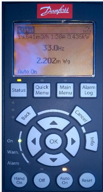
Parameterization is manually with LCP 102, but only table for senseless can be uploaded via Danfoss MCT 10 program. You can parameterize it completely with Danfoss MCT 10.
