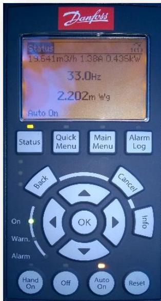
Parameterization is manually with LCP102, but only table for senseless can be uploaded via Danfoss MCT 10 program. You can parameterize it completely with Danfoss MCT 10.
