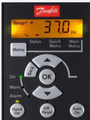
Parameterization is manually with LCP111 and it is installed to each frequency controller. It can be moved to other controllers on site, so you need just one.
